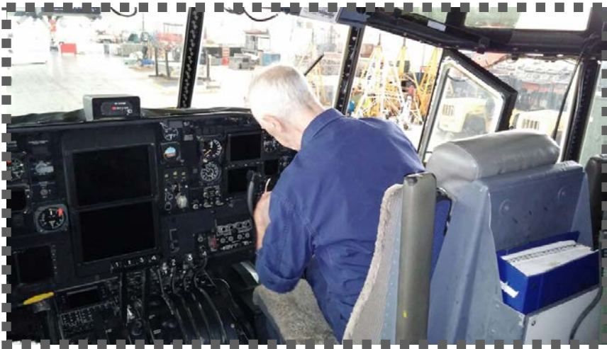
Removing the GPS from the co-pilot position.
